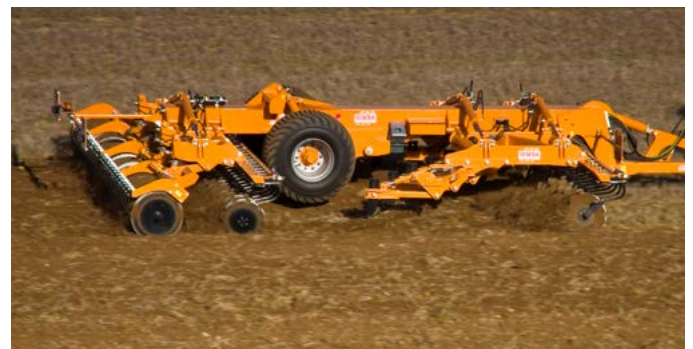
Figure 23. Typical high disturbance, deep non-inversion mixing action
