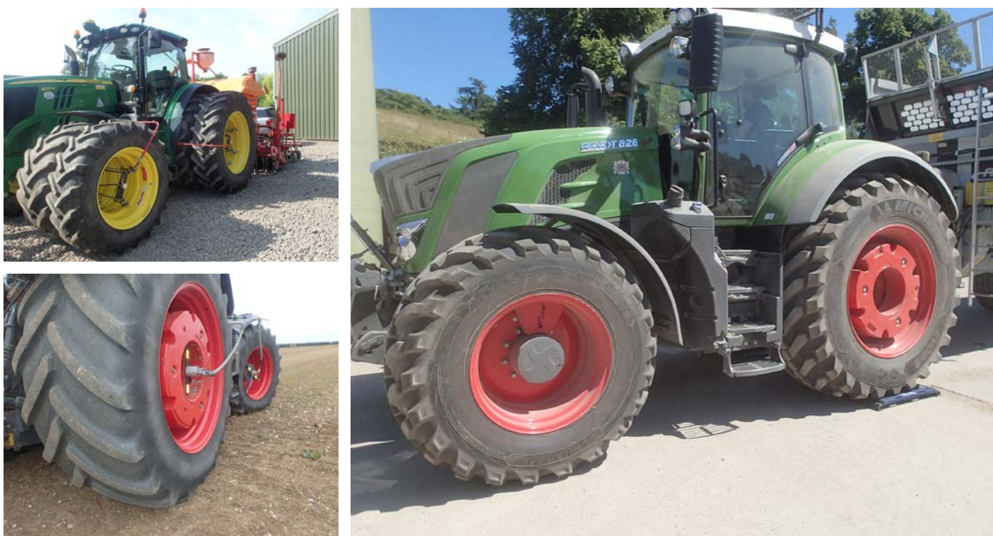
Figure 8. Retro-fit central tyre inflation system (CTIS) options (left, top and bottom) and original-fit, fully integrated CTIS (right)
