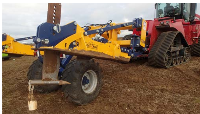
Figure 1. Mole drains are formed by dragging a 'bullet' followed by an expander through the soil to form a circular semi-permanent channel
