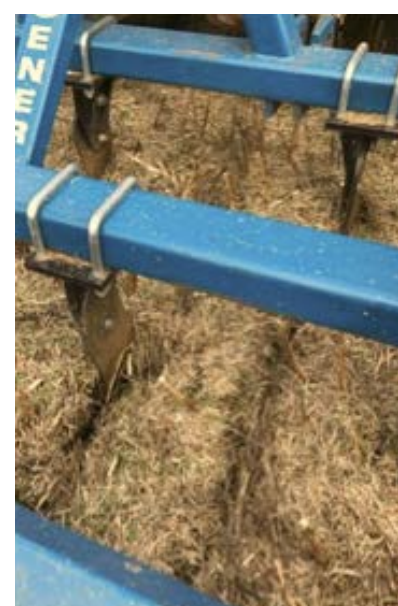
Figure 14. Geometry of loosening parts and minimal surface disturbance (left). Sufficient lift to create vertical fissures is needed at the problem depth. Low rake angles minimise surface disruption and heave, provided lift height is adequate for fissure creation. Sideways inclined legs (right) can also minimise surface disturbance, provided operational speeds are appropriate
