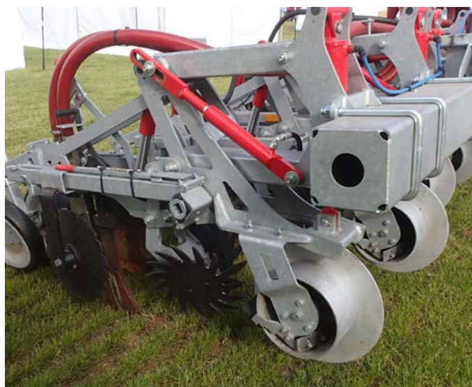
Figure 30. Example of leading and side-border discs, with leading residue manager wheels
