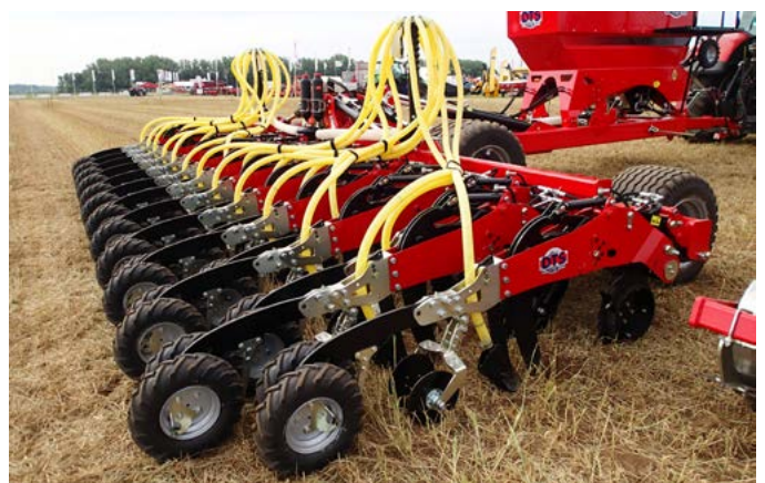
Figure 29. Dedicated all-in-one strip tillage drills
