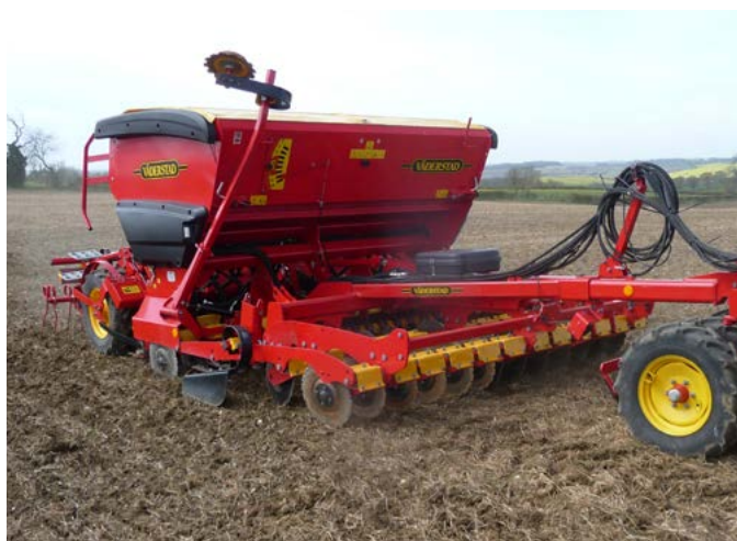
Figure 31. Combined structuring and drilling (top) and cultivator drill used as a direct drill with cultivation elements raised clear of work (bottom)
