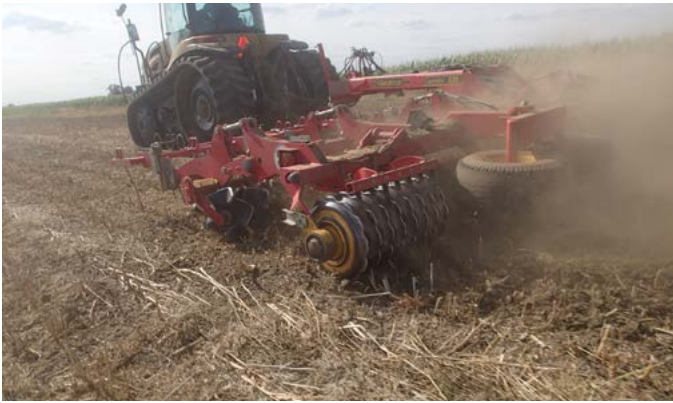
Figure 26. Wave-type discs on a shallow non-inversion cultivator
